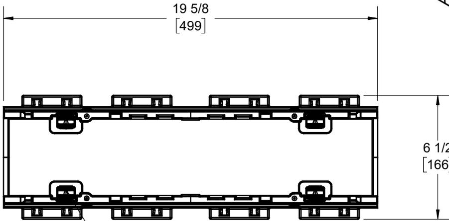
PRO-SNAP CONNECTION TO CHANNEL ONLY FOR ATTACHING DI RAIL
