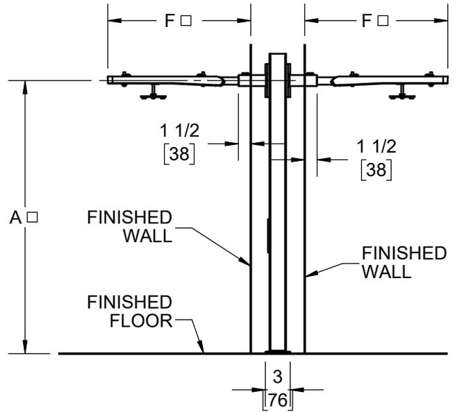
JOSAM RECOMMENDS FEET BE SECURED TO FLOOR WITH 1/2" BOLTS AND ANCHORS BY OTHERS
