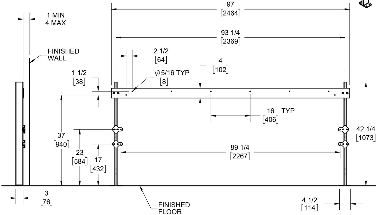
JOSAM RECOMMENDS - FEET BE SECURED TO FLOOR WITH 1/2" BOLTS AND ANCHORS BY OTHERS
