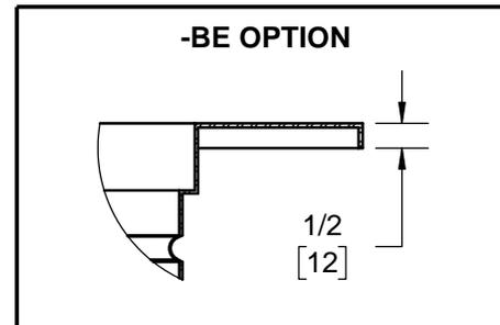
OUTLET O.D. FITS CLOSELY WITH I.D. OF NO-HUB CAST IRON PIPE
